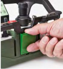
**Change-over battery AK5** for power supply without memory effect, based on NiMH technology, providing continuous operation time of up to 16 hours, can be replaced quickly if needed As a true all-rounder the radio transmitter TMS-56 can be used for different tasks. In the field of wireless controls this transmitter is the best choice for crane controls, among others, no matter if it is a single, a tandem or a taking-over system.
